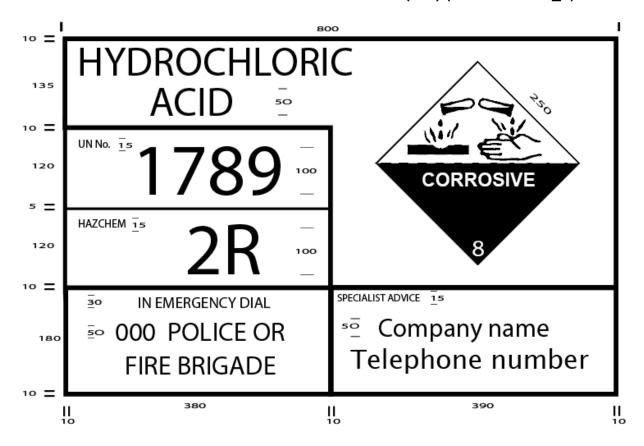
This **Transport Emergency Information Panel (EIP)** has black text on a white background with the specified class label as per the Australian Code for the Transport of Dangerous Goods by Road & Rail (ADG Code).
