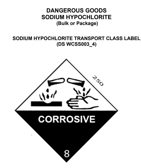
This **Transport Class Label is** as per the requirements of the Australian Code for the Transport of Dangerous Goods by Road & Rail (ADG Code). Material: Metal or Plastic – 250mm x 250mm.
