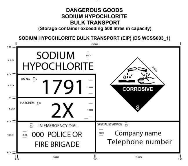
This **Transport Emergency Information Panel (EIP)** has black text on a white background with the specified class label as per the Australian Code for the Transport of Dangerous Goods by Road and Rail (ADG Code).
