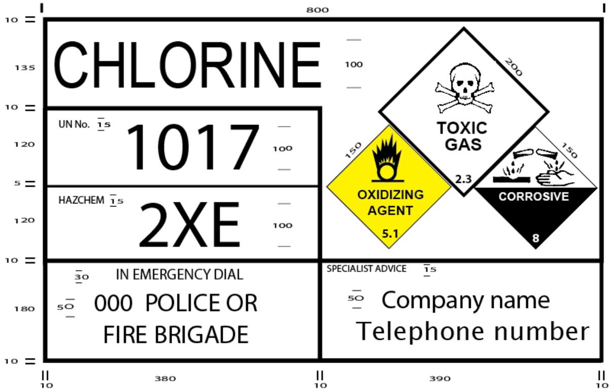
This transport **Emergency Information Panel (EIP)** has black text on a white background with the specified division and subsidiary hazard labels as per the Australian Code for the Transport of Dangerous Goods by Road & Rail (ADG Code).
