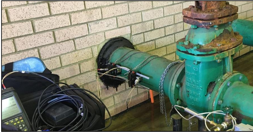
Figure 19: A Strap-on ultrasonic flow meter being used for pump testing
