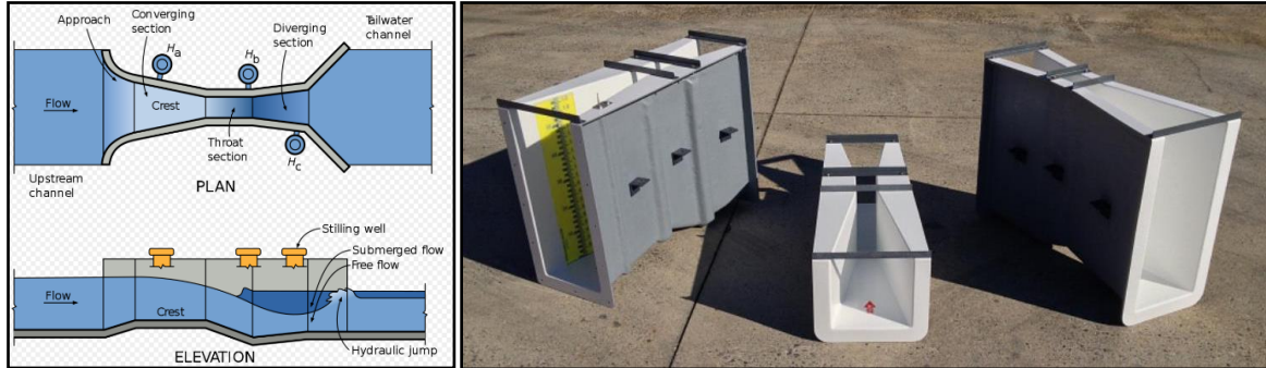
Figure 8: Flume measurement, (left) Parshall flume design, (right) fabricated examples
