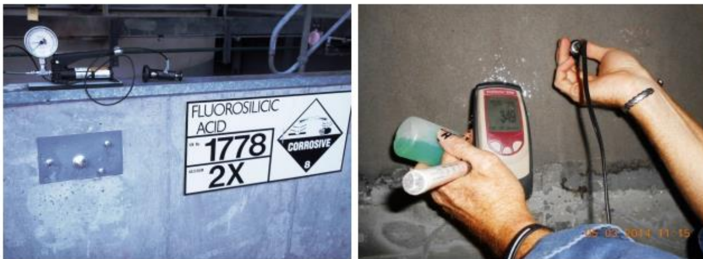
Figure 6– Typical adhesion test equipment, DFT testing Positector gauge
