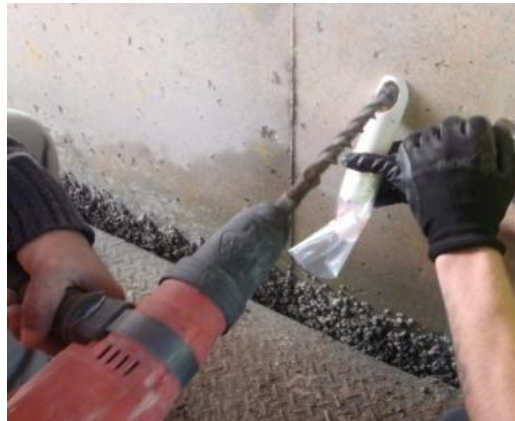
Photo 27 - Example of collecting powder sample for laboratory analysis
