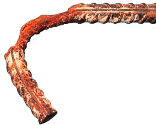
Photo 22 - Classification 5G. Severe localised attack; Rest of the bar suffered lesser uniform attack.
