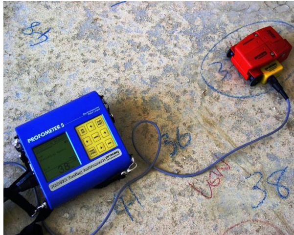
Photo 28 - Concrete cover meter inspection on the floor.
