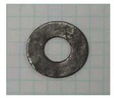
• Lead washer 22mm (OD) x 9.6mm (ID) x 1.3mm thick Store MMR - 20002
