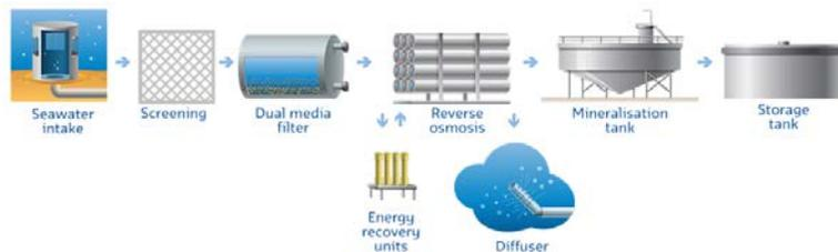
Figure 14. Typical desalination treatment process
