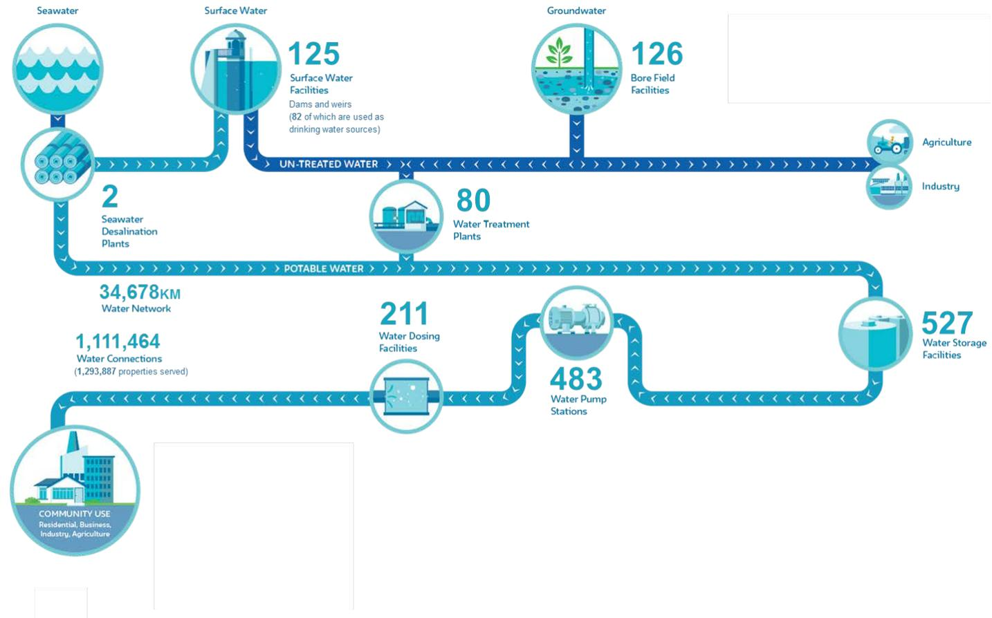
Figure 2. State-wide drinking water assets and generalised layout – as at 30 June 2018
