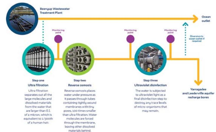
Figure 16. Advanced water treatment process
