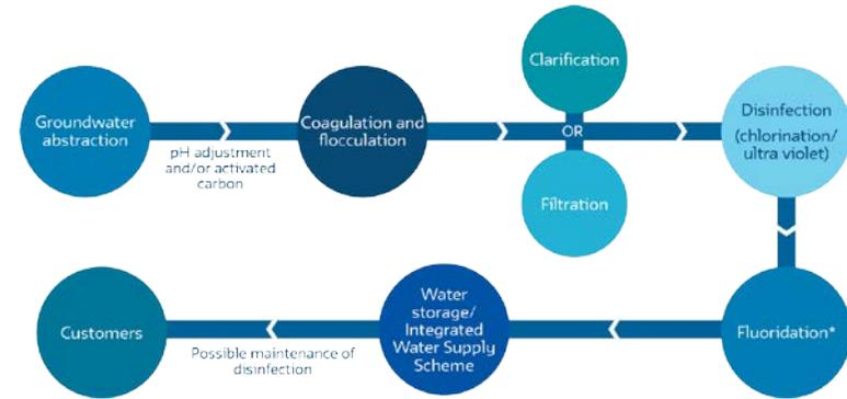
Figure 20. Example of a more complex treatment process
