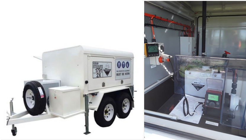
Figure 24: Mobile chlorine dosing unit
