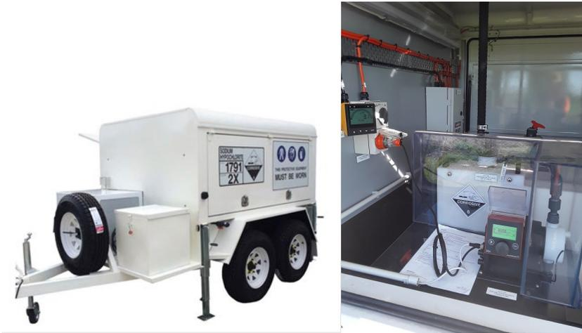
**Figure 24: Mobile chlorine dosing unit**
