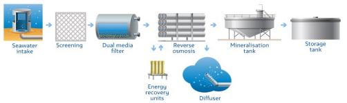
Figure 24: Typical desalination treatment process
