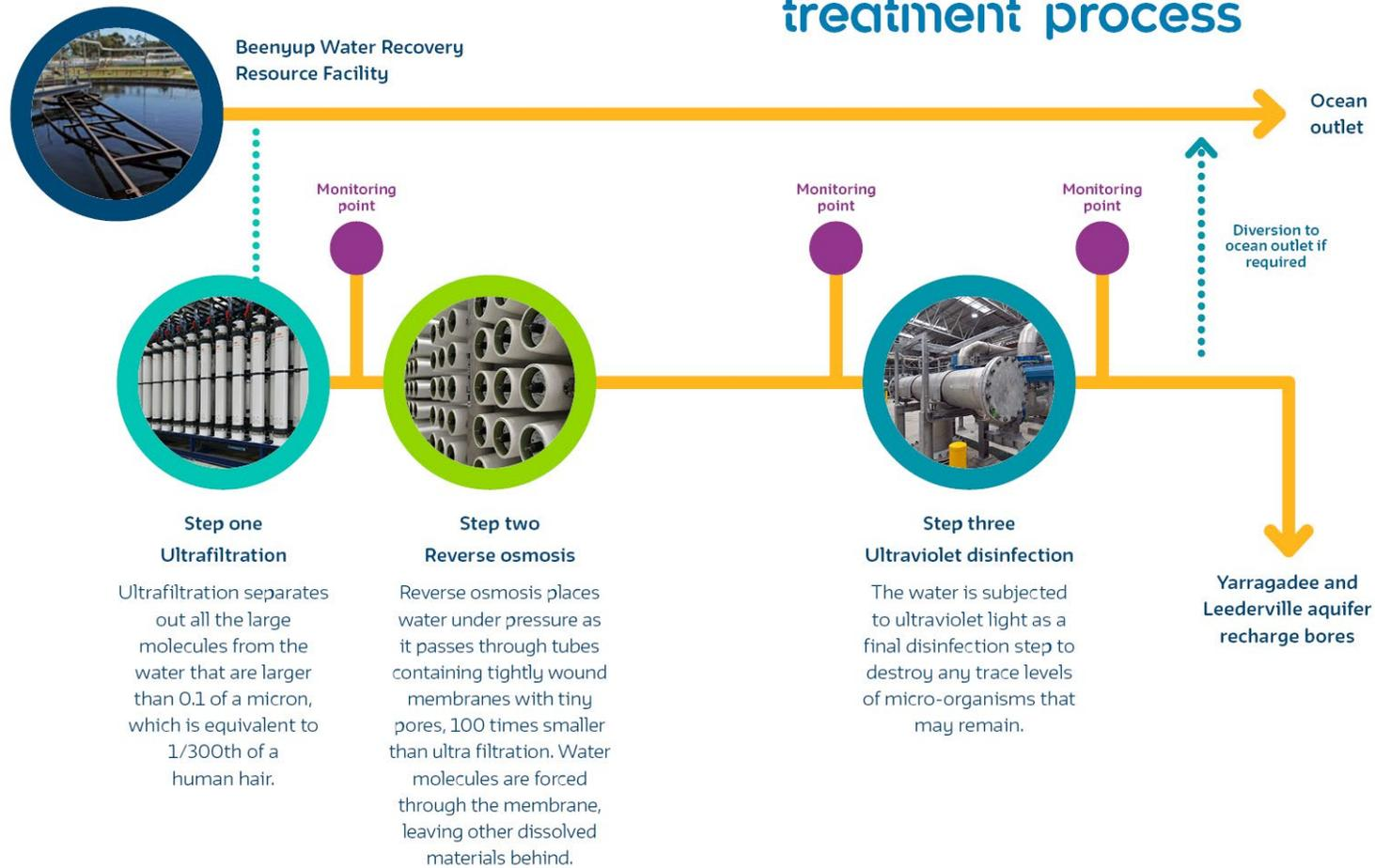
Figure 25: Advanced water treatment process
