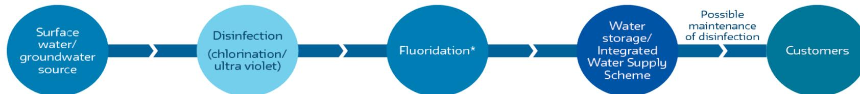
Figure 22: Example of a basic water treatment process \*(see *Fluoridation* section for those towns that have fluoride added to their water)
