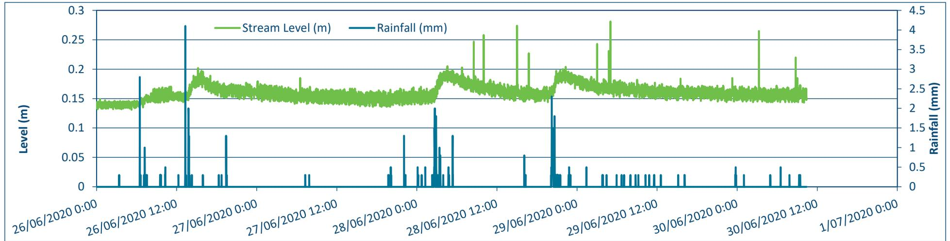
Figure 19. Ten Mile Brook Dam main feeder creek level and rainfall.
