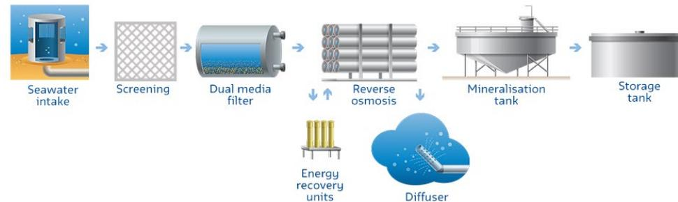
Figure 24: Typical desalination treatment process
