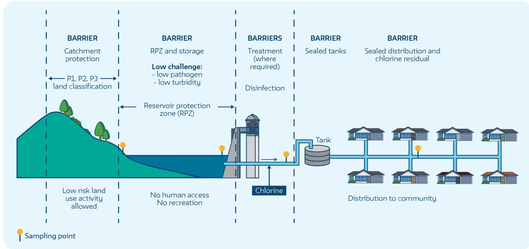
Figure 17: Surface water catchment – showing source protection and additional multiple barriers
