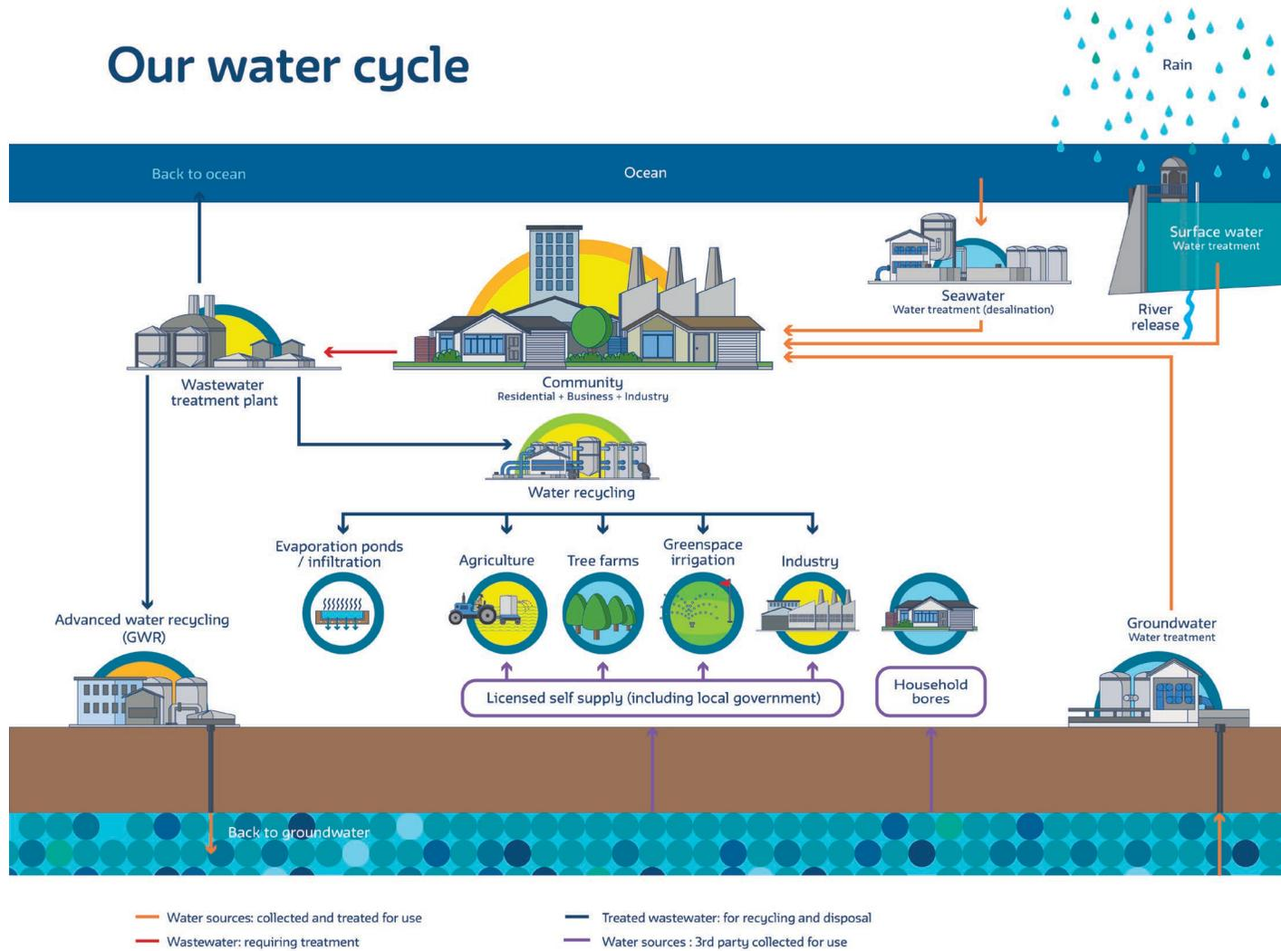
Figure 11: Groundwater replenishment in the water cycle
